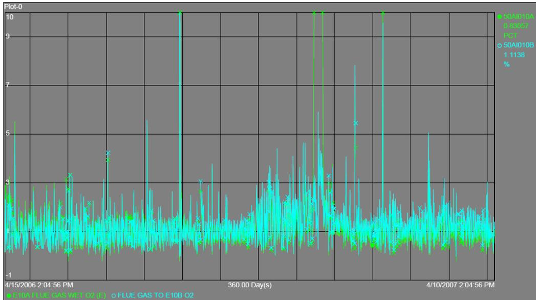
**FIG. 3) ACTUAL DCS TRENDS FROM AN FCCU REGENERATOR SHOWING OXYGEN PERIODIC OXYGEN DEFICIENT READINGS.**
