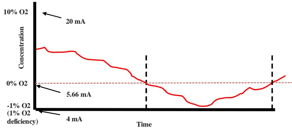
**FIGURE 2) REPRESENTATION OF A DCS TREND WITH AN ELEVATED ZERO, PERMITTING AN OXYGEN DEFICIENCY INDICATION.**
