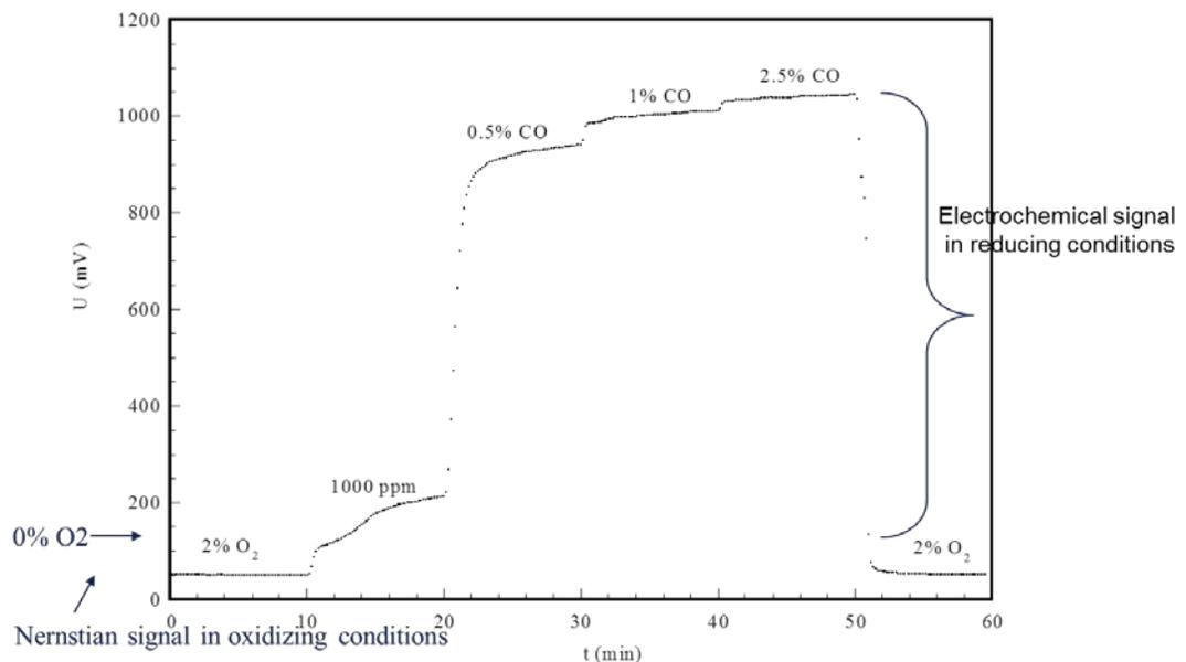
**FIGURE 1) Z<sub>R</sub>O<sub>2</sub> CELL OUTPUT IN OXIDIZING AND REDUCING CONDITIONS.**
